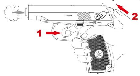
Please make sure to empty the CO2 cartridge by the venting hammer after the game in the right procedure. Check out the BLE-PM2 CO2 cartridge installation instruction online.
